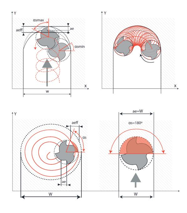
Circular milling vs. Full-slot milling
