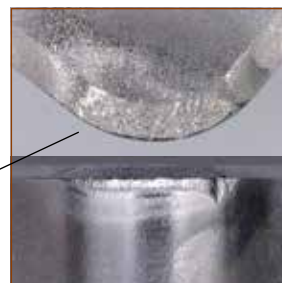
BNS8125 (After cutting 9,0 km)
