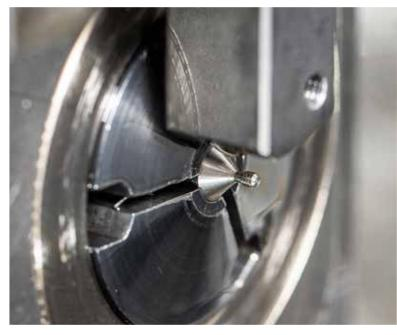
Turning the M1.6 x 0.35 thread with the S274 system.
