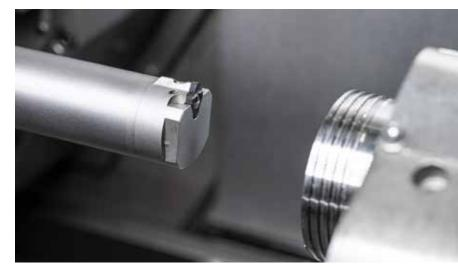
HORN relies on the 117 system for broaching the spline.
