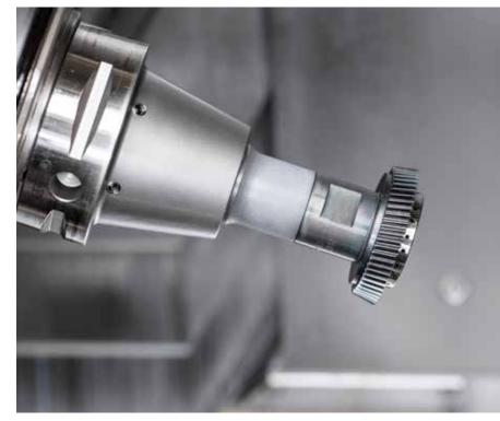
More than 40 variants of the precision tools are in use at Neugart for producing gears from module 0.5 to 2.
