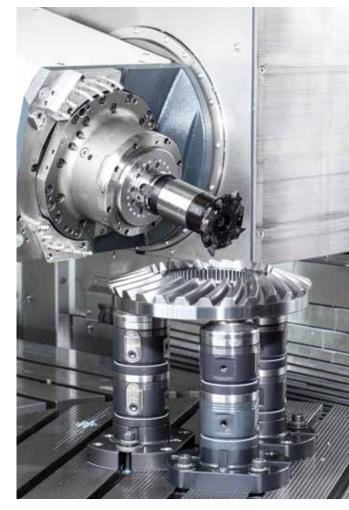
HORN developed the M279 milling system for economical roughing of cyclo-palloid gears.
