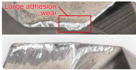
After drilling 900 holes
