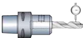
Set-screw types runout 0.02 – 0.04 mm
